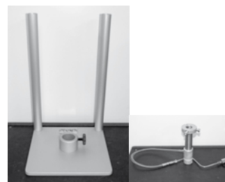
Vacuum stand & pipe for nylon bag technique
